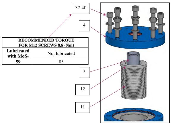
6.8 - Fit the spacer (mark 5) into its place taking care to fit it into its lodging of the piston (mark 3).
