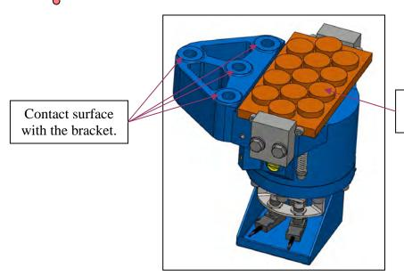
Contact surface between the linings and the disc.
