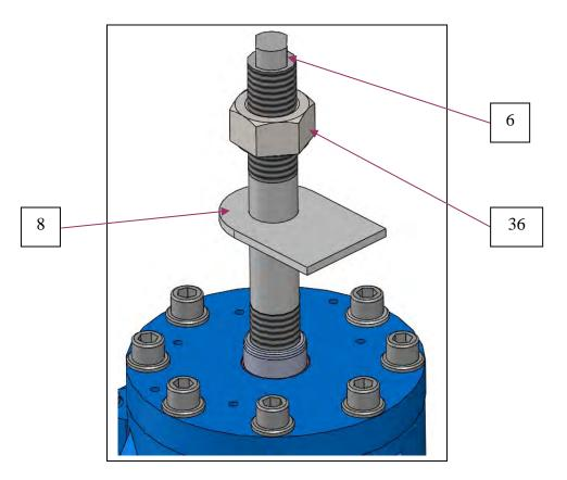
7.4 - The spring lock is still compressed, which means that if the cover (mark 4) is removed now the springs would exert stress that might be dangerous.
