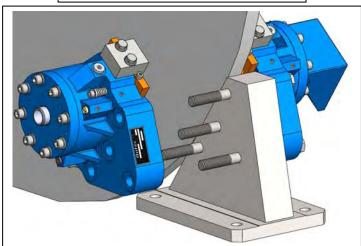
7.9 - Without any hydraulic pressure, loosen the 8 screws with their washers (mark 37-40), which fasten the cover (mark 4) of the brake.
