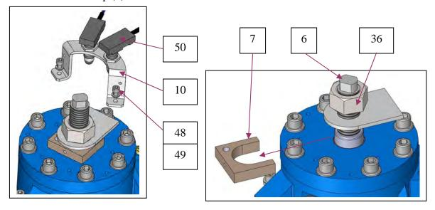
4.1.4 - Screw or unscrew the adjustment screw (mark 6) until the distance between the lining and disc is 1 mm. This is called the airgap. The 1 mm must be measured with a gauge.
