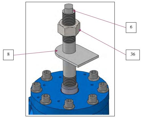
6.4 - The spring lock is still compressed, which means that if the cover (mark 4) is removed now the springs would exert stress that might be dangerous.
